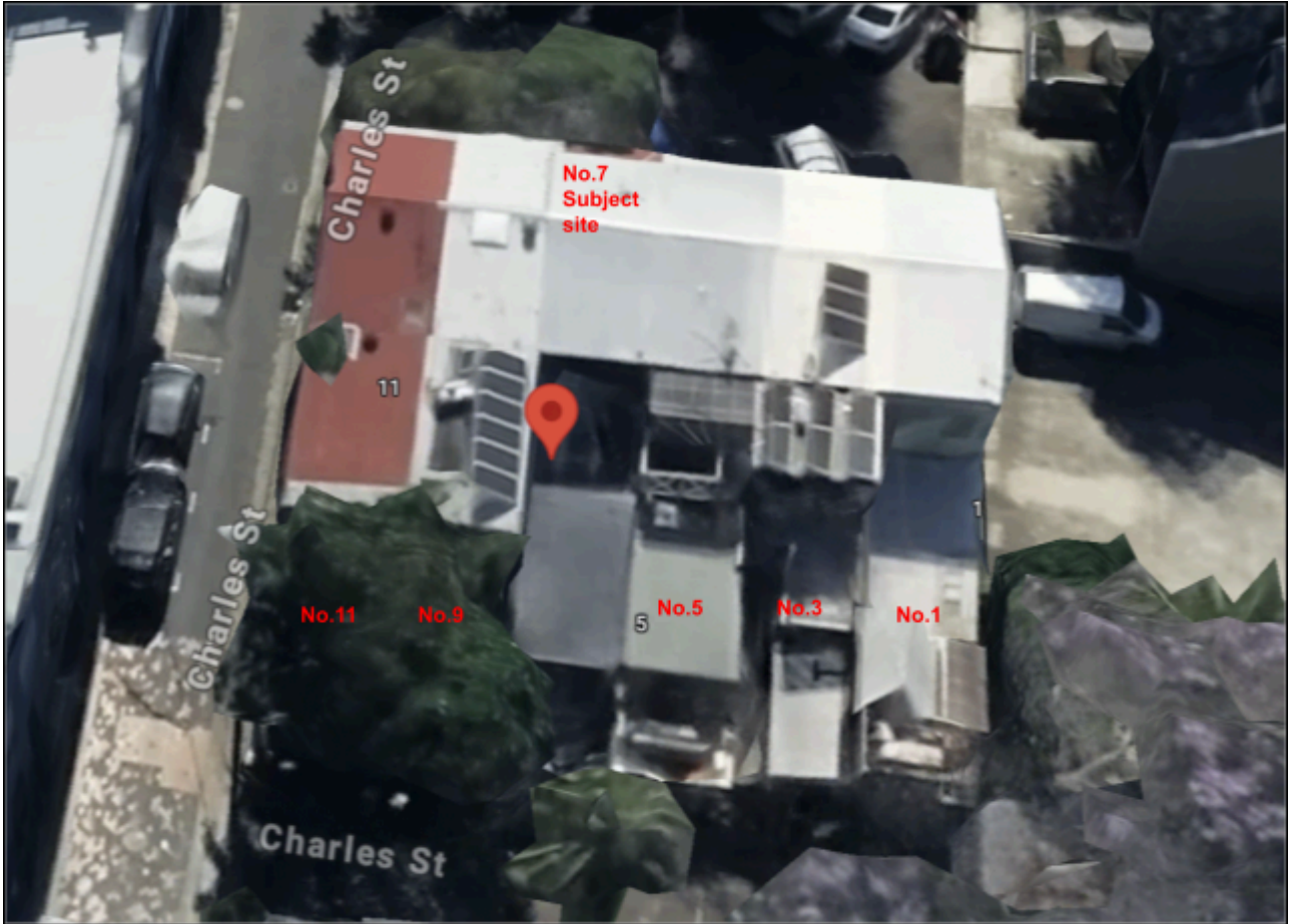
Fig 3 - Demonstrating the consistency of the proposed built form with neighboring dwellings. Nos 9 and 11 have a consistent first floor rear setback to that being proposed. Nos.1, 3 and 5 have ground floor rear setbacks consistent with the subject site.
